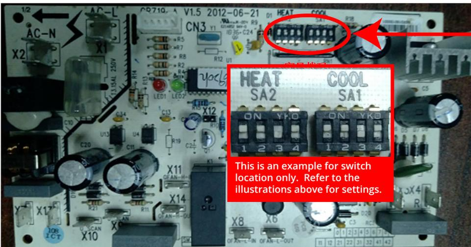
Location of Dip Switch on Air Handler Main Board
