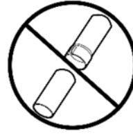
Do not crimp service valve connector when pipe is smaller than connector
