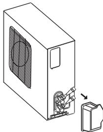
2. Do not remove the plastic seals from the outdoor unit piping connectors and corresponding refrigerant pipes (line set to be attached) until immediately before you connect them.
