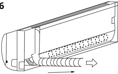
3. Now, you will need to lightly tape the refrigerant piping and drain pipe together in a bundle, using electrical tape, making sure that the drain pipe is at the bottom. **DO NOT** tape the ends of the piping (connectors). Refer to Fig 4.7 and the image below for the correct orientation of the piping when taping.
