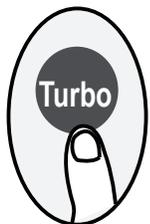
**When the TURBO button is pressed while the unit is in COOL mode,** the unit will blow cool air with highest fan setting to speed up the cooling process.
